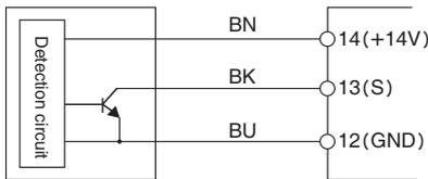
4) PNP transistor output connection diagram:
